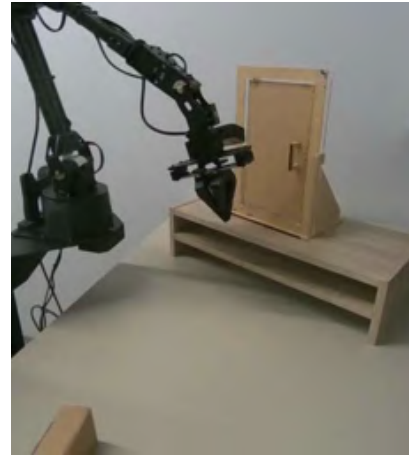
Figure 8. Real-world setup. A WidowX arm attempts to open a door that can either be pulled or pushed open.
